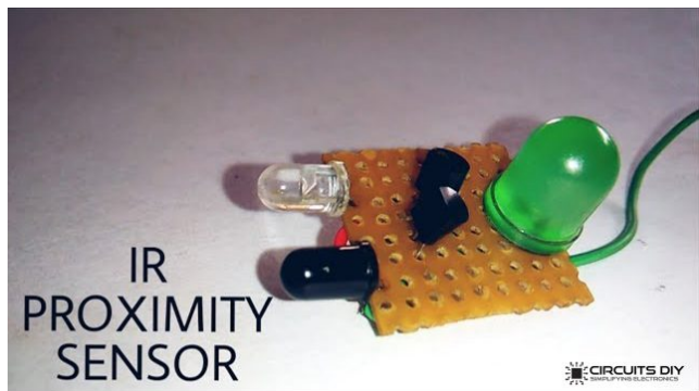
Infrared Proximity Sensor Using Transistors - IR LED
