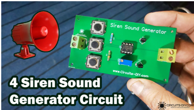
4 Siren Sound Generator using UM3561 - Police Ambulance Sound
