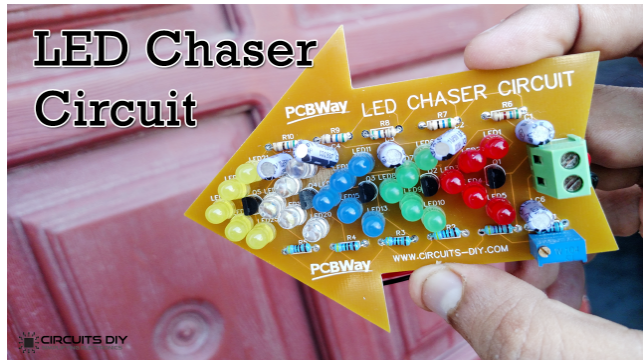
LED Chaser Circuit using Transistors - Electronics Projects
