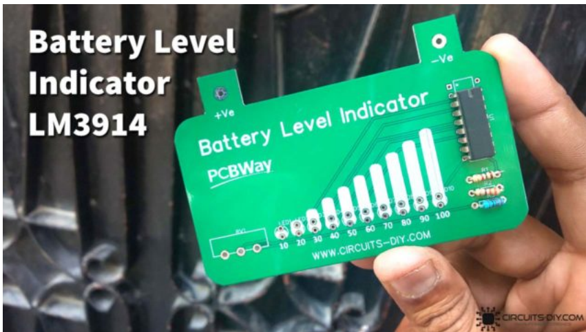
Battery Level Indicator using LM3914 - Electronics Projects
